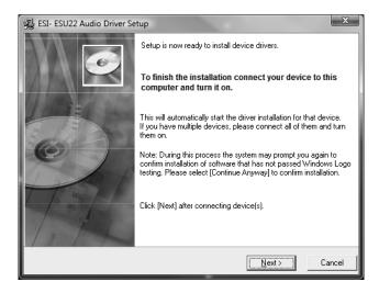
You can now finally click *Next* on the *ESI ESU22 Audio Driver Setup* dialog. The installation is now finished. To confirm this, please check if the ESI icon is displayed in the taskbar notification area as shown below.
