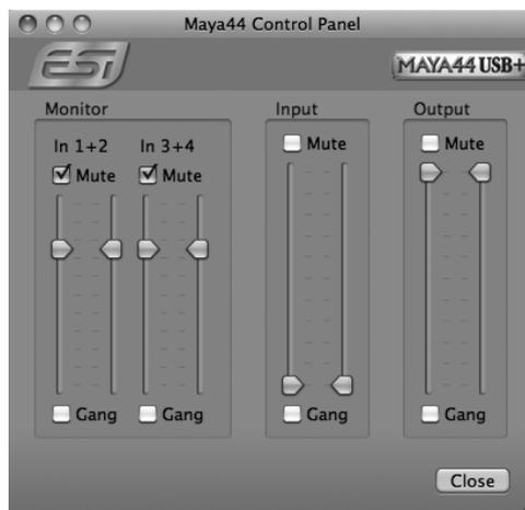
You can control the input monitor level, the input level and the output level with the faders in the control panel.
