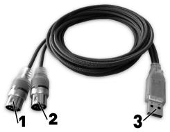
MIDIMATE eX features two separate MIDI connectors (1 and 2) and a USB connector (3). The MIDI connectors are labeled 1 and 2 and each of them can connect to the MIDI input of a device (then they work as an output) or to the MIDI output of a device (then they work as an input). The USB connector connects to the USB port of your PC or Mac.
