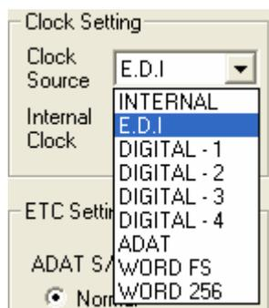
**Internal:** Use the internal clock inside EX8000.
