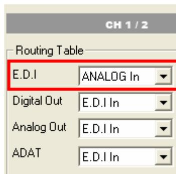
Please have a look at the following audio routing table that shows you all the audio routing options of EX8000 when connected to the MaXiO PCI host card.
