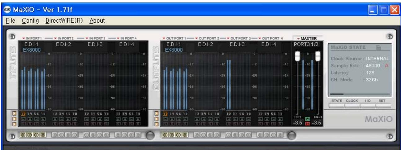
In many typical setups you would use output 1/2 of the first port (e.g. the first EX8000) as master output. Via the monitoring buttons (see below) you can then mix all signals to this stereo output.
