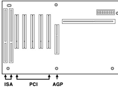
*typical PC motherboard slot configuration*
