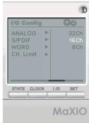
**CH. Limit:** The *CH. Limit* setting allows you to limit the maximum number of channels that are transferred via the PCI bus. If you select *32Ch*, all 32 input and 32 output channels are active at the same time. If you select *16Ch*, only the first 16 input and the first 16 output channels are active, if you select *8Ch*, the first 8 input and the first 8 output channels are active. The lower the setting will be, the lower the PCI transfer generated by the MaXiO PCI host card will be.
