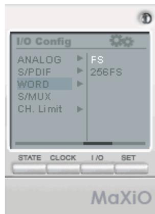
**Word:** this setting allows you to define if you want to send out a standard Word Clock (*FS*) or a Super Clock (*256FS*) signal via the Word Clock output of the M.D.I connection, e.g. the M.D.I breakout cable.
