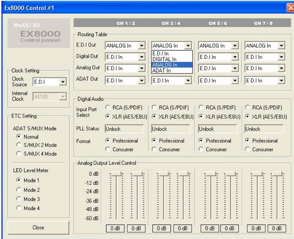
**Clock Setting:** Defines the system clock of the specific EX8000 unit.
