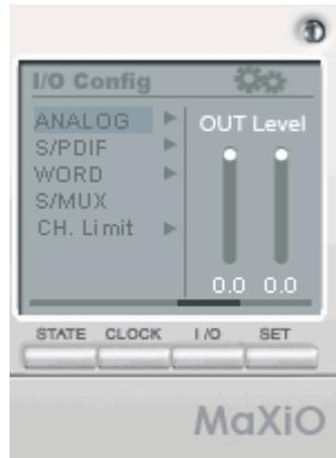
**Analog:** This where you adjust the analog output level of the analog output channel of the MaXio PCI host card. This analog output is only available when you have connected a device to the M.D.I port with analog outputs (such as the MaXio 032 breakout box).
