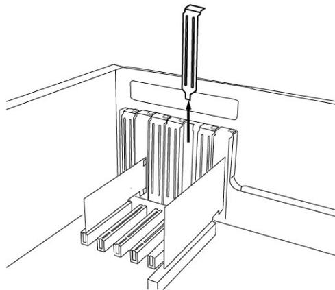
*removing the PCI slot faceplate*
