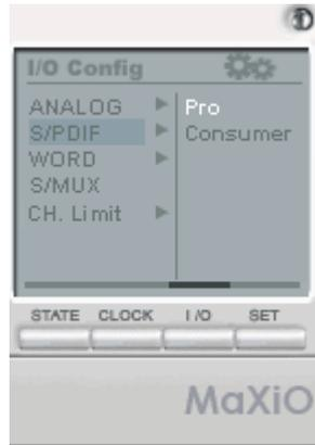
**S/PDIF:** this can be *Pro*, which means that actually an AES/EBU signal with the ‘professional’ status bit set is transferred via the S/PDIF I/O of the MaXio PCI host card (via the M.D.I connection, e.g. the M.D.I breakout cable), or it can be *Consumer*, which means that normal S/PDIF signals are transferred.
