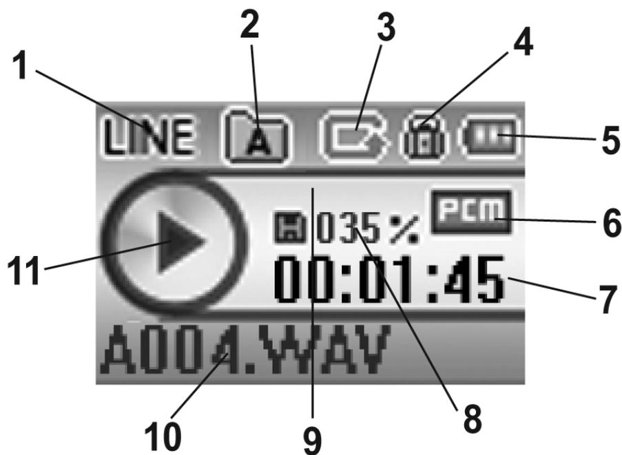
1. shows the current input source for recording: *INT* (internal stereo microphone), *WIDE* (internal stereo microphone with higher sensitivity for wider rooms / areas), *EXT* (external mono dynamic microphone) or *LINE* (external stereo line input).
