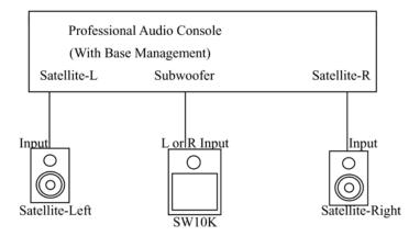
In a 5.1 or a 7.1 setup, the other surround speakers will also be connected to the source directly although the diagram does not show that. If your source device is only stereo and / or does not have its own base management, the satellites are connected to the outputs on the right side of the back panel of SW10K eXperience using balanced XLR cables. Refer to the following diagram:
