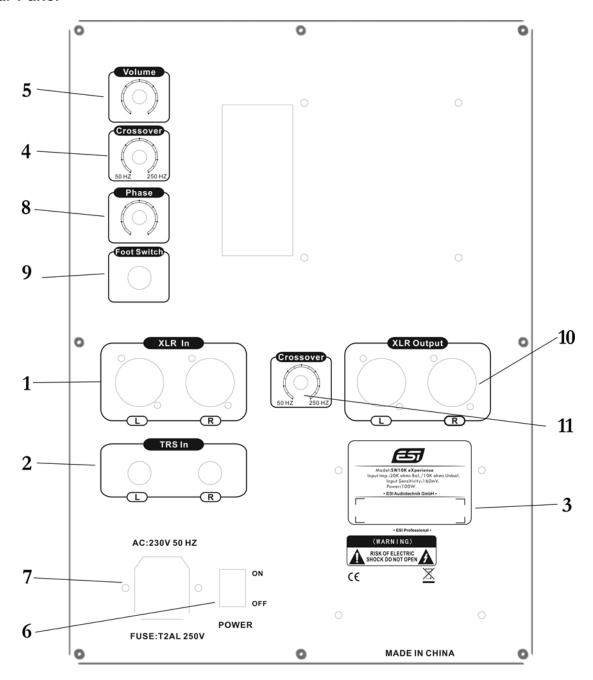
**1. XLR inputs** – these connectors accept balanced XLR input connections. The XLR input is wired like this:
