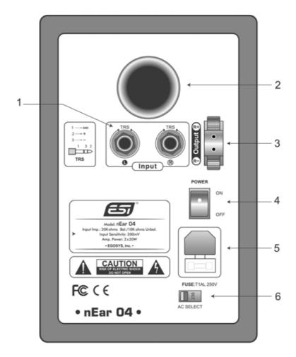
**1. TRS input** – these jacks accept TRS input connections, either balanced or unbalanced. For balanced connections, a 3-conductor TRS plug is necessary. The TRS input is wired like this:
