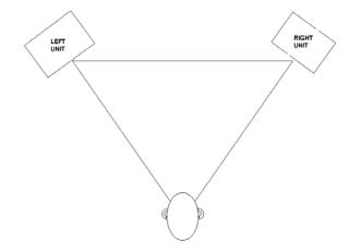
The height of the units, more precisely the top of the woofer, is recommended to be at the ear level of the listener. Keep in mind that in a typical monitoring environment, you are sitting in front of your workstation. Refer to the following diagram:
