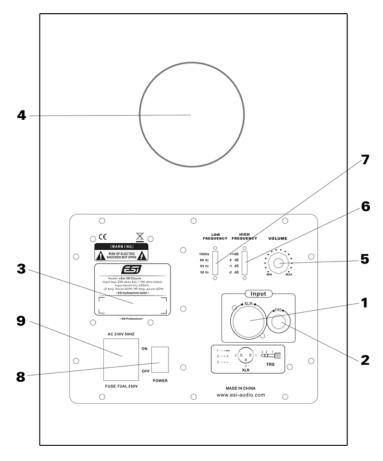
**1. XLR input** – this connector accepts balanced XLR input connections. The XLR input is wired like this:
