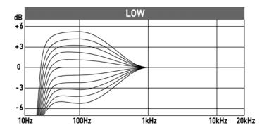
When set to 0 (middle position), the whole frequency response is optimised, i.e. as linear as possible. Make sure that each speaker has exactly the same settings.
