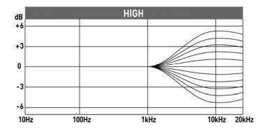
When set to 0 (middle position), the whole frequency response is optimised, i.e. as linear as possible. Make sure that each speaker has exactly the same settings.
