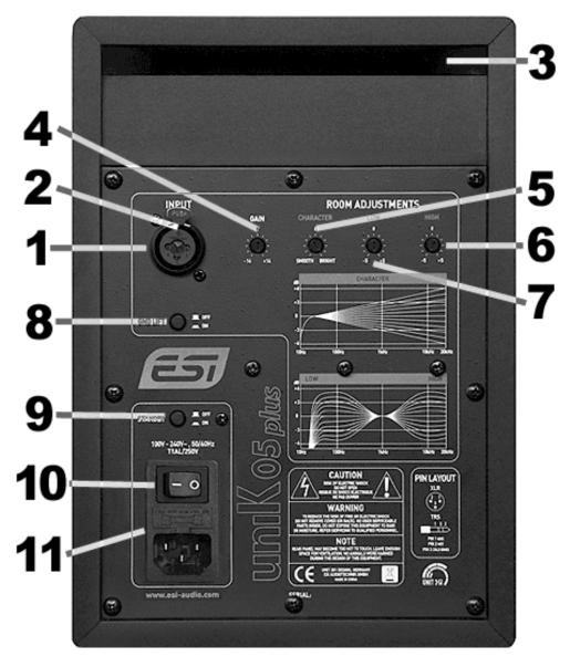
**1. XLR input** – this connector accepts balanced XLR input connections (typically with a +4dBu level). XLR input is wired like this:
