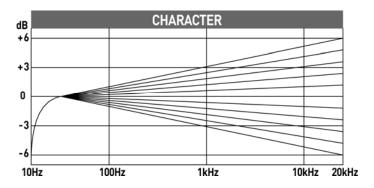
When set to 0 (middle position), the frequency response is optimised, i.e. as linear as possible. When the value is tilted upwards, the higher frequencies will appear stronger, yet the whole frequency spectrum will match accordingly. When the value is tilted downwards, the high frequencies will appear less strong. It is recommended to adjust the *CHARACTER* first, before you change something on the *LOW* and *HIGH* knobs. Also make sure that each speaker has exactly the same settings.
