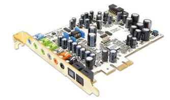
Prodigy X-Fi NRG is a powerful 7.1 channel, 24-bit / 96kHz capable PCIe based soundcard featuring the AKM AK4358 D/A Converter for playback signals with 112dB dynamic range. The combination with a fine selection of high quality condensers and a special circuit design provides perfect sound quality. The OpAmp on the card is installed on a socket, providing the possibility to change it to users preference.
