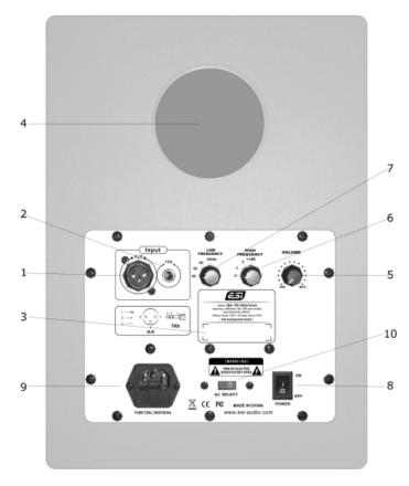
1. XLR input - this connector accepts balanced XLR input connections. The signal of the XLR input is mixed together with the TRS input signal through a balanced input amplifier. The XLR input is wired like this:
