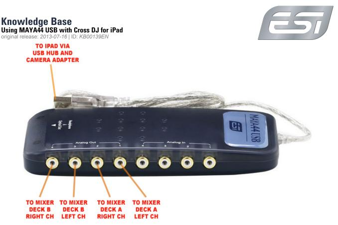
MAYA44 USB has a built-in headphone amplifier, however you cannot use it for monitoring in a DJ application as it sends out always the mixed signal of all channels (1-4). Because of that your monitoring headphone should be connected to your DJ mixer in this setup.
