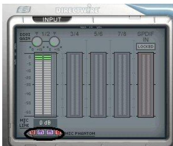
You can control gain from -60dB to +15dB (0.5dB per step) on input ch 1/2. Also, input ch 1/2 supports +12V phantom power microphone. To use the microphone you must change the input level to “M” (microphone) from “L” (line input). After selecting “M”, you can select “12” (12V) on each channel for phantom power.
