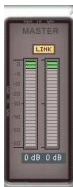
**LINK:** You can control volume of left and right channels independently by deselecting this button.
