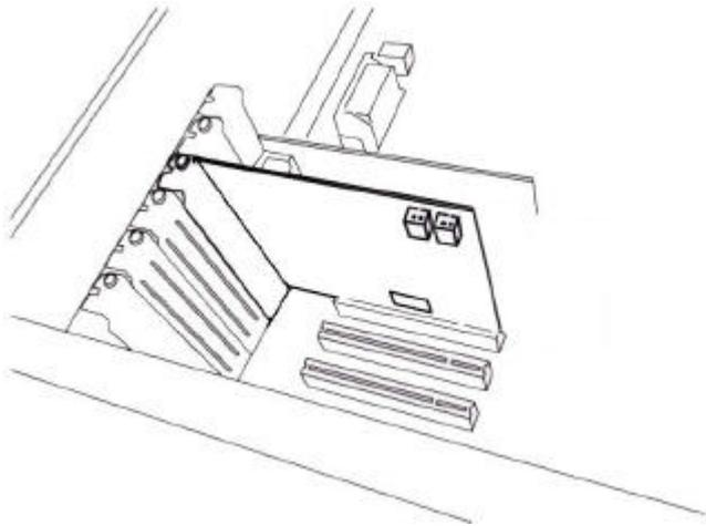
Figure 5. MAYA44 MKII Installed in a PCI slot
