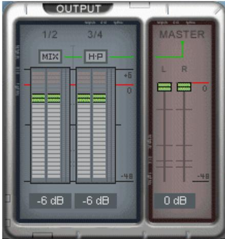
Adjusts and monitors the output levels of each audio channel via level faders and meters. If you click the Headphone icon on the Output 3/4 level fader, the output port 3/4 is switched to a headphone jack. MAYA44 MKII features a high-fidelity headphone amplifier.
