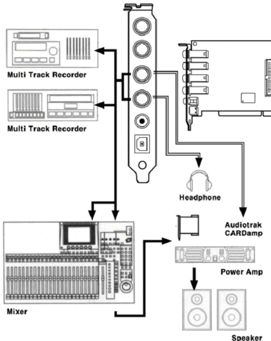
4. Digital Output(Coaxial, Optical) can be used to record your wave output, MP3 files, or wave files directly to an MD, DAT, or CD Recorder. You can connect SPDIF compatible devices such as an MD, DAT or CD recorder to transfer audio data with minimal signal loss.
