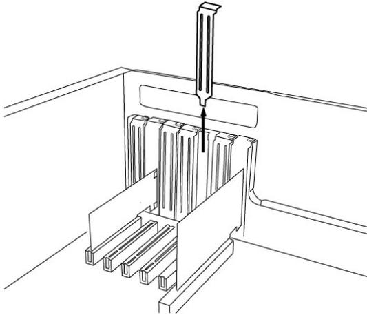
Figure 4. Removing the PCI Slot faceplate
