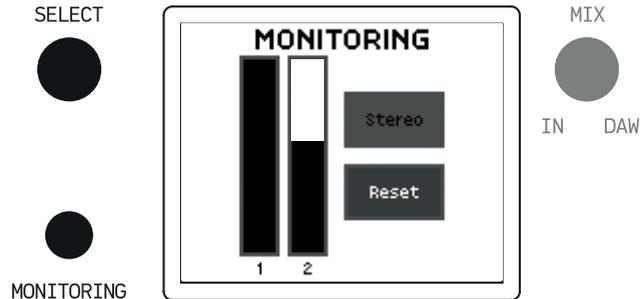
The MONITORING view screen is intended to be a visual representation of each of the volume levels for each of the direct monitoring signals. This Advanced Direct Monitoring functionality is quite unique as you can create a special direct monitoring mix, perfect for even the most special recording and monitoring situations. No matter if you record microphones or guitars or synthesizers, anything you need to monitor via your studio monitors or headphones can be setup directly on the hardware.
