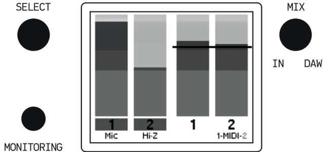
The standard view of the LCD screen shows the active signal levels for input channels 1 and 2 on the left half of the display area and the playback levels (DAW signal) for channels 1 and 2 on the right half of the display area as level meters. The level meters are separated into different colors. The red color on the top means that the signal is probably too loud and possibly clipping while an optimal signal level is typically orange. The green area indicates that a signal is present.
