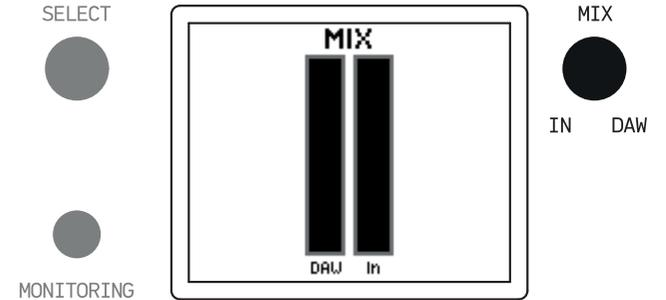
The MIX view that is displayed when you use the MIX encoder, shows a visual representation of the output/playback (DAW) and input (IN) signals.
