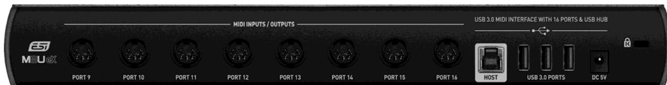
The rear panel features MIDI ports number 9 to 16, next to the USB **HOST** connector which is used to connect M8U eX to a computer. Right of it are the 3 **USB 3.0 PORTS** that allow you to connect and use any other USB device with your computer (i.e. USB keyboard, USB memory, USB dongle, etc.) and a **DC 5V** connector to connect M8U eX to the included power supply. To the very right there is a standard laptop lock connector that you could use to prevent the unit from being stolen.
