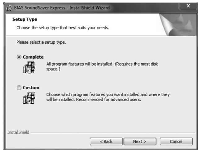
The next dialog asks you to proceed with the installation process by clicking *Install*. Now the files will be copied to your system (which may take a while) and the finished installation will be confirmed with the final dialog that you can close by clicking *Finish*.
