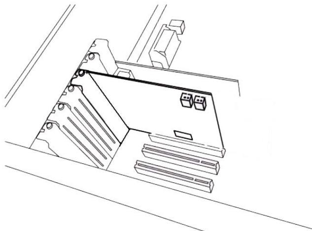
*Figure 5. Prodigy 7.1 HiFi installed in a PCI slot*
