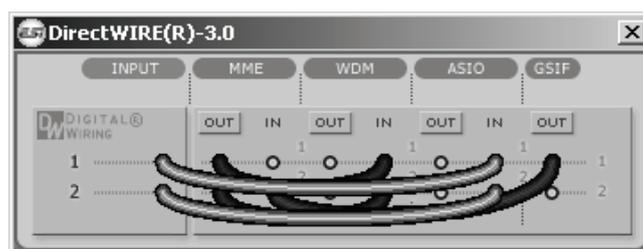
The number on the row represents the input or output port. The columns represent ins and outs (on and off) of the respected drivers. Patch the virtual cables from one point to another as you drag your mouse point.
