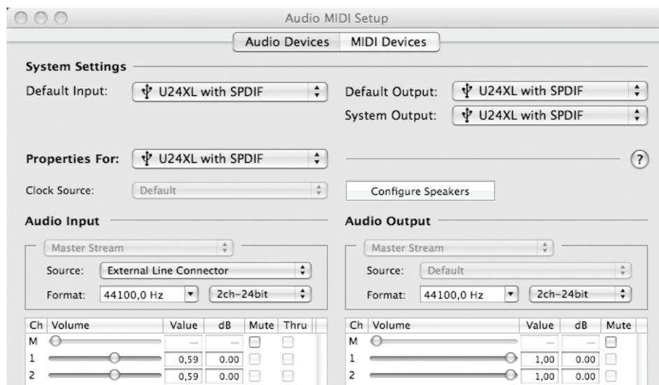
While audio production and editing applications usually provide an option inside their preferences to select U24 XL as recording and playback device, many general standard applications such as iTunes for example are usually accessing the *Default Output* device, selectable in the *Audio MIDI Setup* dialog.
