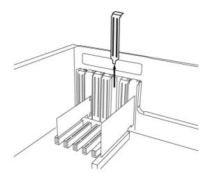
Next, put the Waveterminal 192X & 192L PCI card into the slot and make sure it is placed in the slot correctly. The card will fit into your slot and then tighten the screw.
