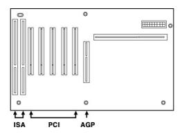
There are 3 kinds of slots in most of recent computers. The PCI slot is most common and is used for different types of devices from the soundcard to the modem. Usually, the PCI slot is the white-colored slot. The ISA slot is used in older computers and it is marked with a black slot. The AGP slot is only for the video card and is the most recent type of slot. It is marked with a brown slot and is located close to the CPU. It will be not too hard to find the PCI slot for Waveterminal 192X & 192L.
