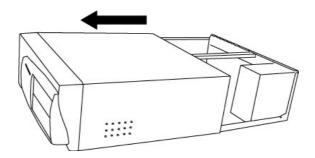
4. To avoid possible static shock to the computer parts, discharge it by touching the computer case or something grounded. We recommend you to use an antistatic device such as an anti-static wrist band.
