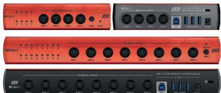
Each unit is a USB 3.0 device (USB 2.0 legacy mode available). They can be bus-powered or powered with an included wall-wart power supply. When plugged in, each unit become a powered 3-port USB 3.0 hub (rear-mounted ports).
