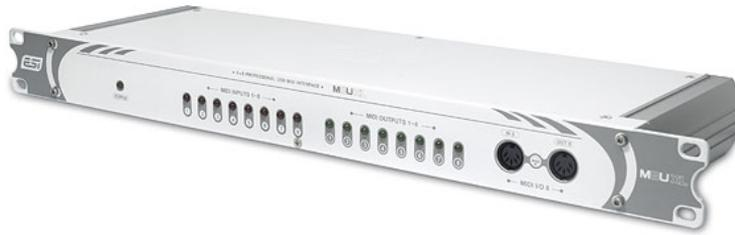
M8U XL offers maximum MIDI connectivity with 8 independent MIDI inputs and 8 independent MIDI outputs, providing 128 MIDI channels - all via a single USB 2.0 (or USB 1.1) connection to your PC or Mac.
